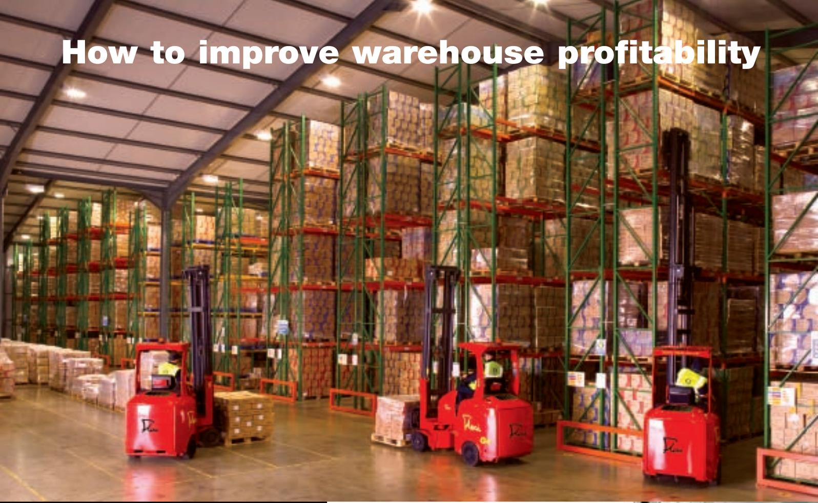
**FLEXI works in just 1642mm (euro)\* or 1762mm (ISO)\* aisle widths - liberating a potential 30% more warehouse capacity compared with conventional reach trucks.**
