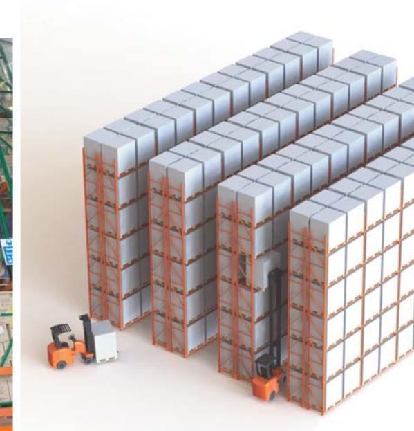
**RediRack narrow aisle racking is a very good space-saving option for warehouses with limited space, providing maximum storage, density and efficiency which can free up to 45% of the floor space when compared to a wide aisle scheme. Each pallet is individually supported and independently accessible.**
