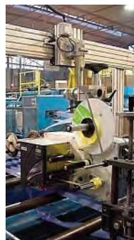
Avery Dennison ALX print engines can apply labels directly to evenly sized products on lines running at steady speeds up to 20 M/minute.
