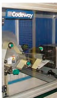
Codeway's Loop Feed attachments for Avery 64 printers feed labels into applicators through a buffer loop.
