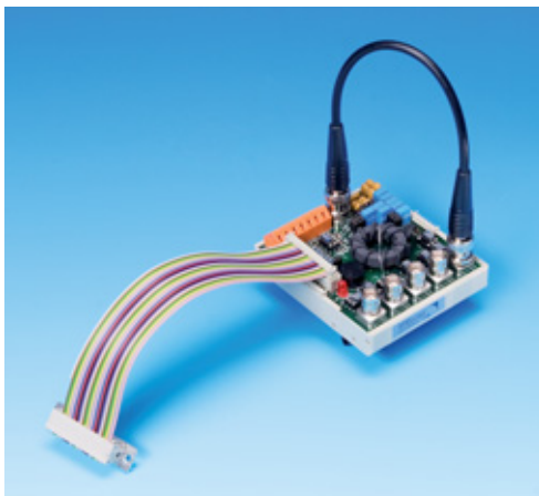
scemtec ® Aerial Multiplexer – Cost effective technically innovative control of RFID aerial systems.
